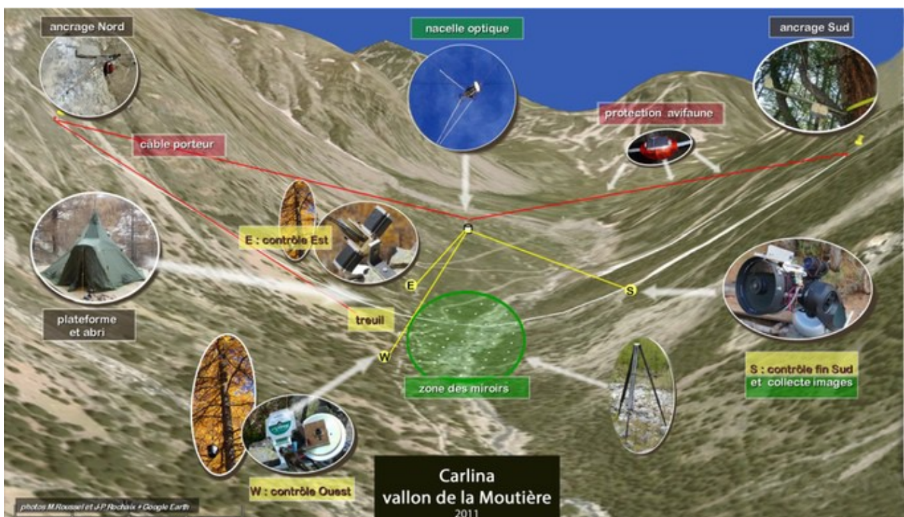
Technical description of Hypertelescope.
