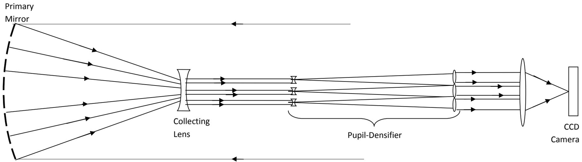
Figure 1: The schematic set-up of Hypertelescope Laboratory Version
